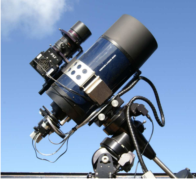
Fig. 1 The BART telescope on its equatorial mount; wide-field camera at the top
