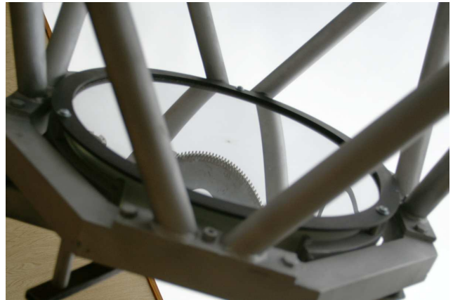
Fig. 5 The primary mirror in the D50 telescope
