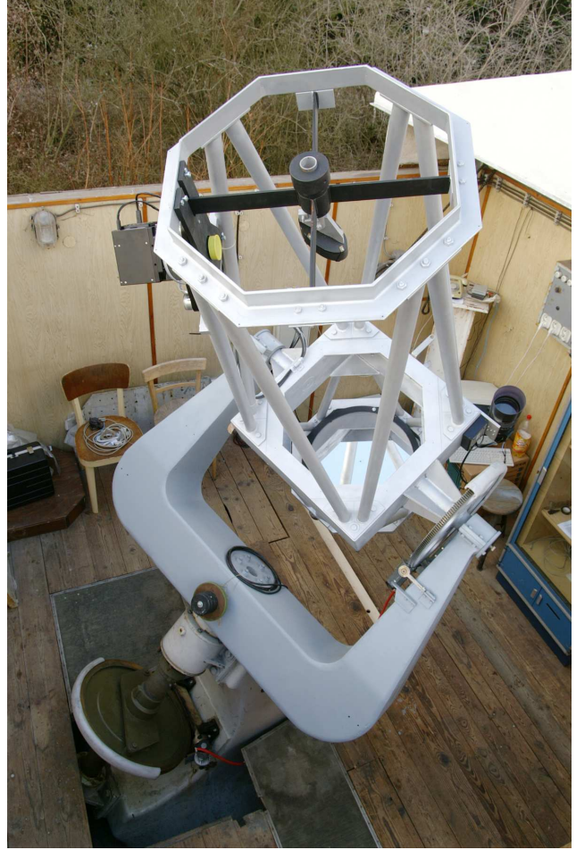
Fig. 4 The D50 telescope with the uncovered primary mirror
