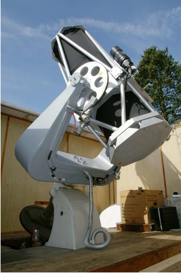
Fig. 2 The D50 telescope on its equatorial fork mount
